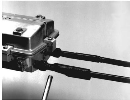
2. Slide the TCS2 cable sleeve back over the connector and begin heating from the connector end. When the sleeve has shrunk around the connector, stop heating for 30 seconds. Push the sleeve up against the closure.
